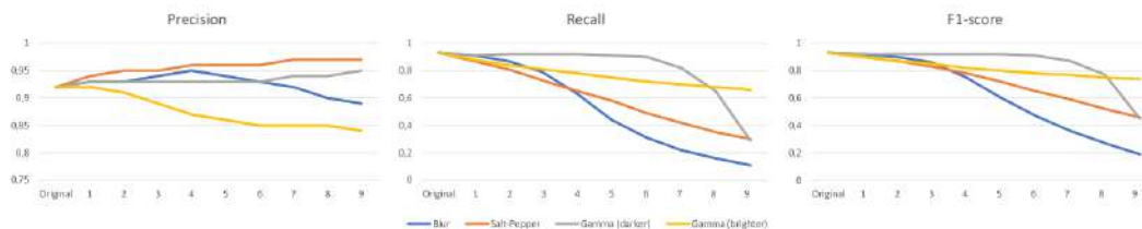
Figure 4.2: Results of the combined model for different degraded versions of the test set by applying blurring, adding salt-and-pepper noise, and applying gamma correction to obtain darker and brighter images. The kernels values for blurring the images are given by 2 \times i + 1 for i from 1 to 9; the probability for adding the salt-and-pepper noise is given by i/100 for i from 1 to 9; the gamma values to obtain darker images are given by 1 - i/10 for i from 1 to 9; and the gamma values to obtain brighter images are given by i + 1 for i from 1 to 9.
