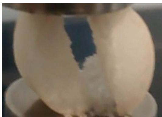
Figura 5.9: Diametral Test. Prensa
