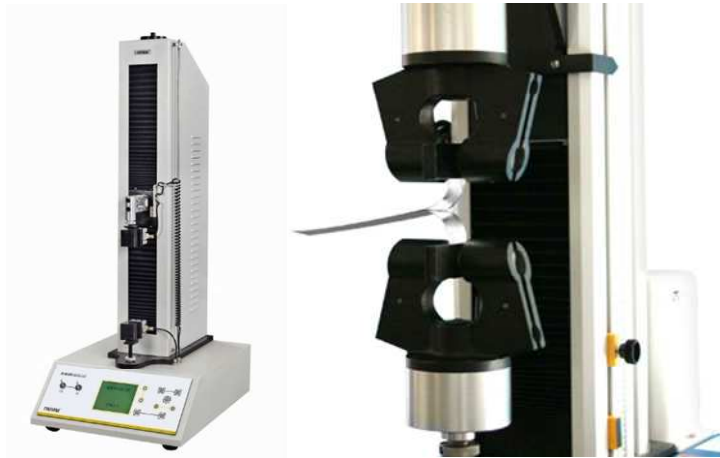
Figure 1.5. Peel Strength Testing Machine. T-peel test.
