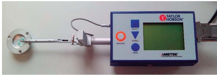
Figure 2.5. Taylor Hobson Surtronic 25 profilometer.
